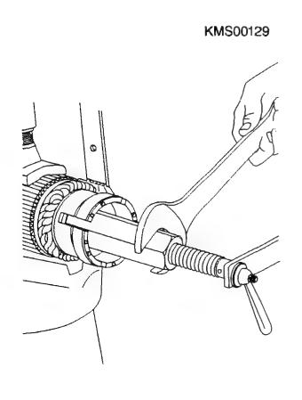
Replacing needle bushing in armature
